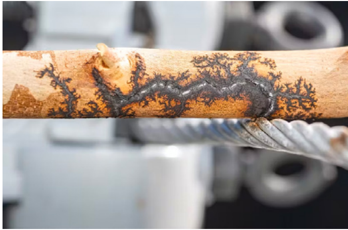
When a tree branch contacts power lines utilizing REFCL technologies, electrical tracking on the branch is seen rather than sustained ignition.
