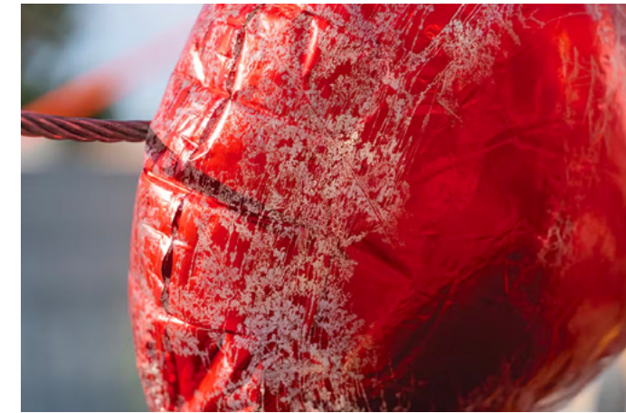
Metallic balloons contacting power lines typically result in an intense arc flash. With a resonant grounded isolation transformer the ground fault energy was reduced to the point that balloons often don't even pop.
