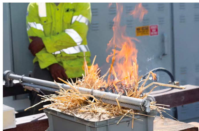
Even low fault currents do not completely eliminate the risk of ignition, particularly when all the current is concentrated into a small contact area. In this case sustained ignition resulted from only 176 mA into a 14.5 inch test cell.
